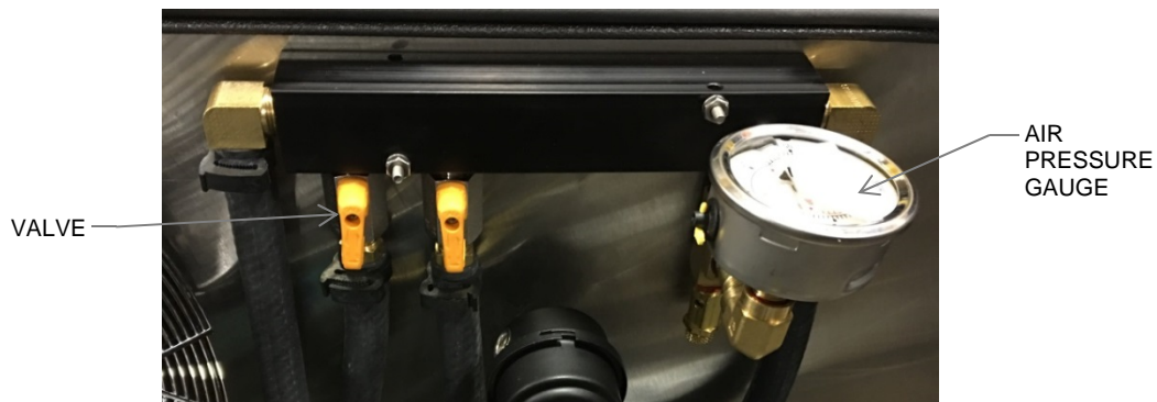
MANIFOLD VALVES SHOWN FULLY OPEN IN THE VERTICAL POSITION
